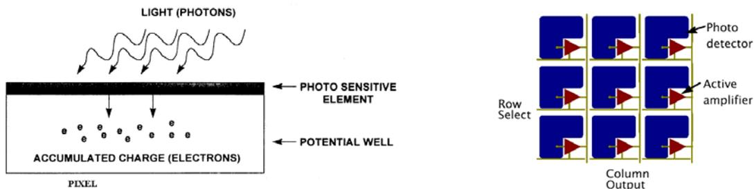
**9.2.1 CCD (Charge-Coupled Device)**
