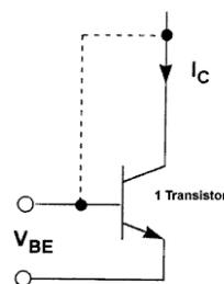
$$V_{BE} = \frac{kT}{q} \ln\left(\frac{I_C}{I_S}\right)$$
