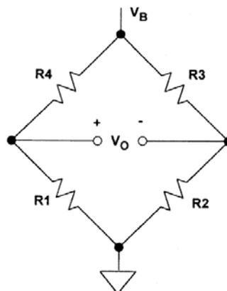
$$V_O = \frac{R_1}{R_1 + R_4} V_B - \frac{R_2}{R_2 + R_3} V_B$$
